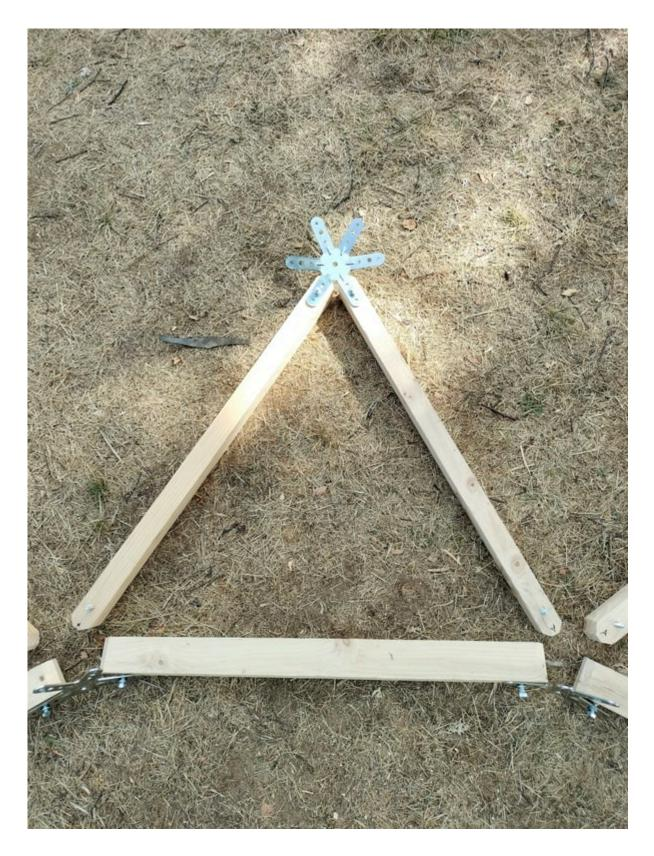
For the last 5 6M connectors in this step, do the opposite: an A-pillar on the left and an X-pillar on the right.
