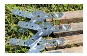
Lay these 5 uprights in a circle with the connectors screwed on top, inserting a large upright between each of them:
