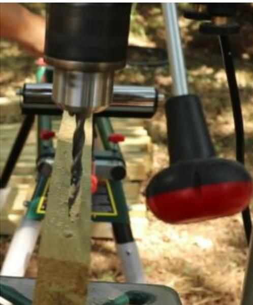
Mark the side where you put the drill bit in: this is the side that will be put against the connectors, as it is the most accurate side.
