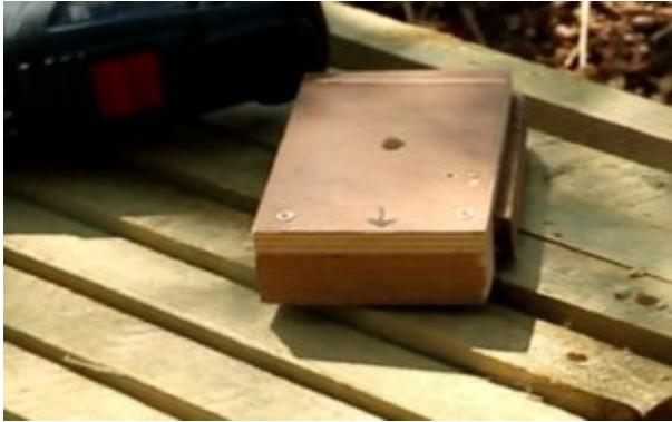
Now complete the 2x25 holes in the studs using your pattern and trying to drill as straight as possible. If you have a drill press, now is the time to get it out.
