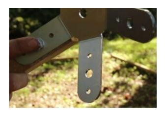
Take the last 6 DOMESTAR 5-way connectors and screw / bolt 1 connector to 6 new posts.
