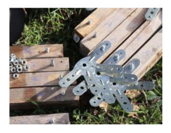
Assemble the 4R and 4L 5x on either side of the B / green / medium uprights.
