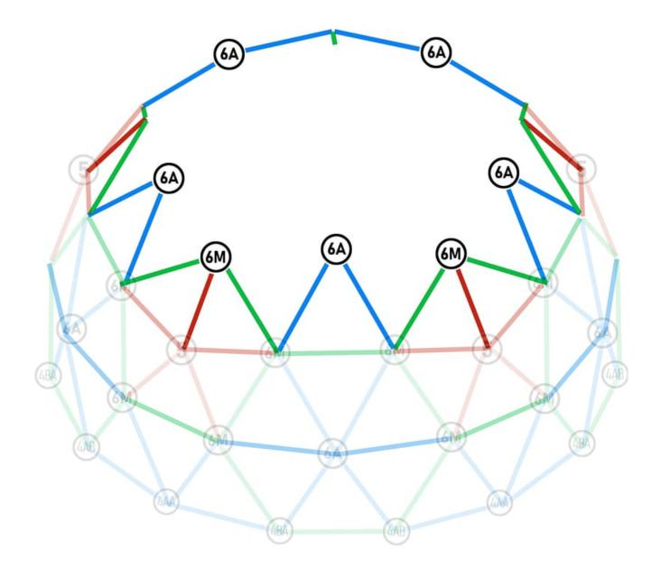
There's a slight difference at this level: instead of just installing 2-legged triangles, we're going to install 3-legged triangles. Look at the plan above: at the 6M connectors we're going to install a C and 2B.
