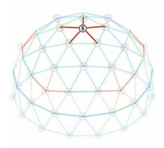
Support the upright during assembly until 3 uprights are assembled:
