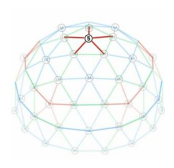
Support the upright during assembly until 3 uprights are assembled:
